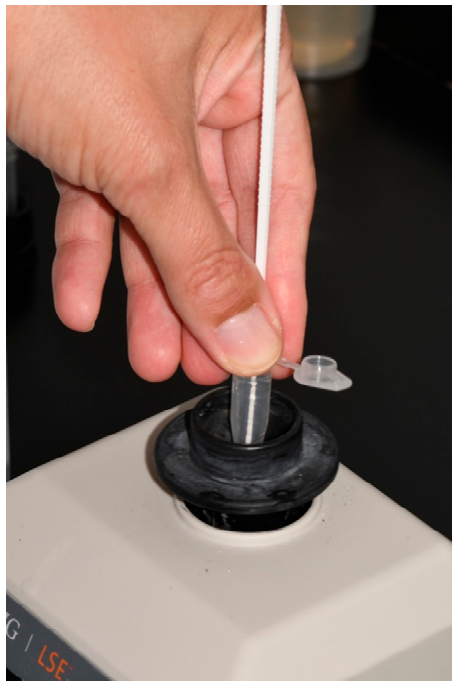
Figure 6. Vortexing of tube containing the infusion and plastic inoculating loop.
